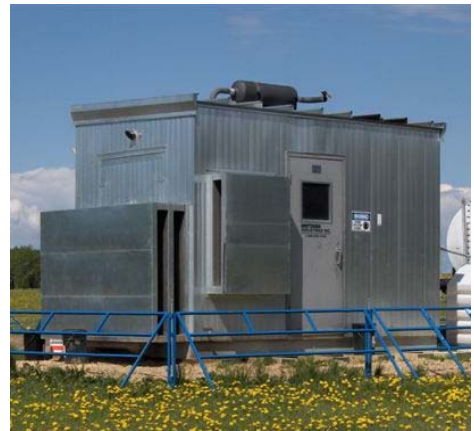
Cummins 5.9 (84HP) Driving a Gardner Denver Enduro 25 Rotary Screw c/w sound suppression package
